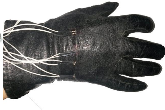
Fig. 2 Glove with sensors for copying healthy hand movement
