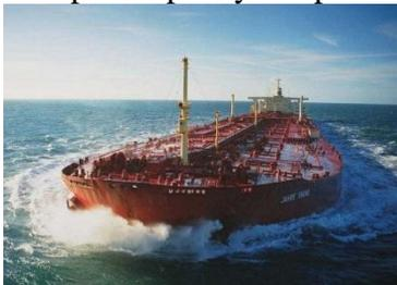
Figure 2 ULCC *Knock Nevis (Jahre Viking)*:displacement 564,763 tdw, length 458.45 m, beam 68.8 m, draft 24.6 m, speed 16 knots
