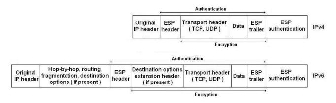
Figure 4.2 – ESP transport mode
