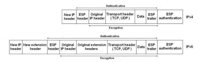
Figure 4.3 – ESP tunnel mode
