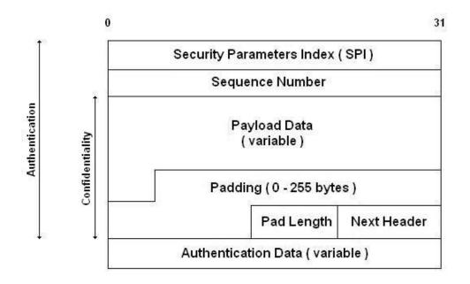
Figure 4.1 – ESP packet
