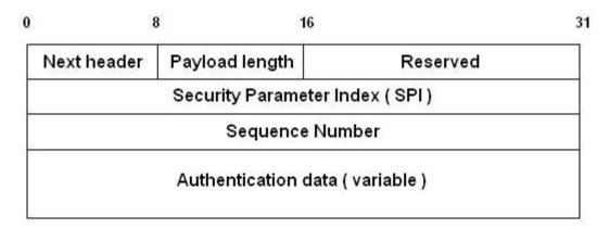
Figure 3.1 – AH header
